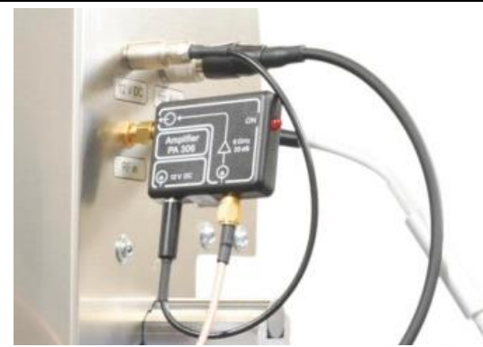
Figure 101: Pre-amplifier power supply cable in the connected state
