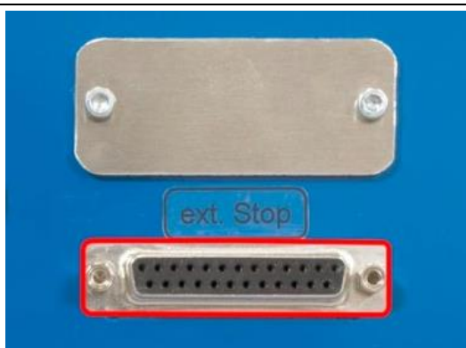
Figure 38: D-Sub port ( ext. Stop )
