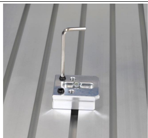
Figure 61: Adjusting the height and angle of the clamping piece with the grub screws
