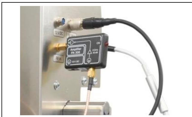
Figure 100: RF measuring cable connected to the pre-amplifier
