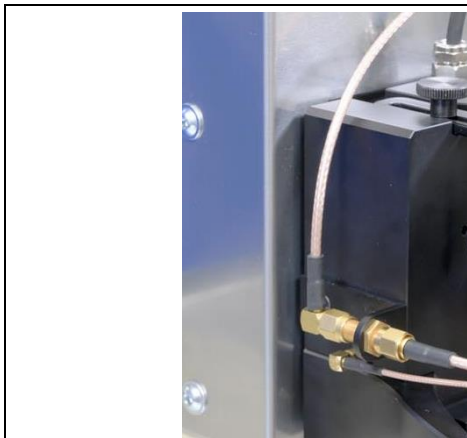
Figure 96: SMA-SMA RA cable connected to the SMA coupling
