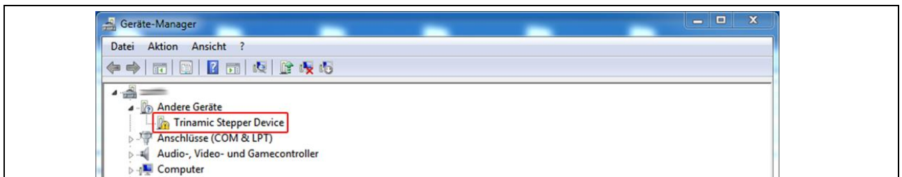
Figure 53: Device manager with the Trinamic Stepper Device entry and an attention sign
