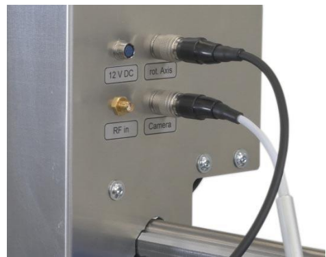
Figure 48: Connecting the HR10 plug of the DM-CAM to the "Camera" connector on the Z-axis tower
