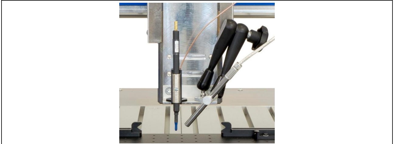
Figure 105: Mounting the near-field probe on the probe holder
