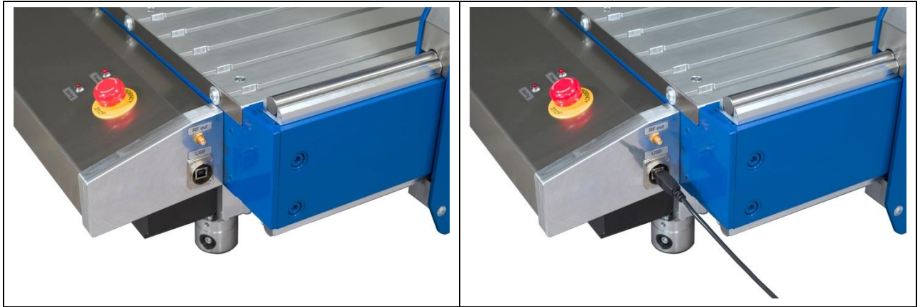
Figure 50: Connecting the USB type B plug to the scanner's USB type B port
