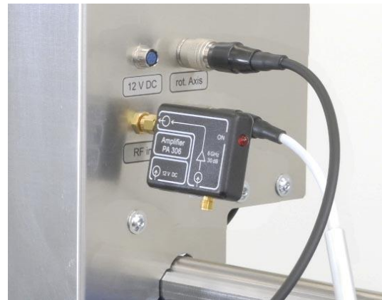
Figure 99: Preamplifier connected to the RF in input on the Z-axis tower
