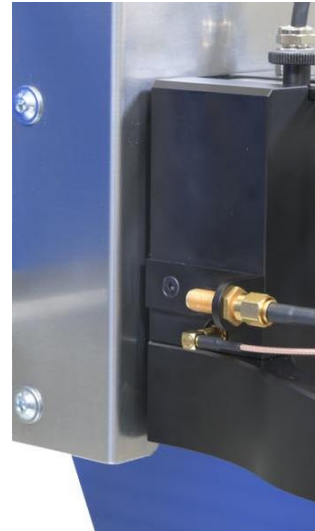
Figure 95: Connecting the RF measuring cable to the SMA coupling
