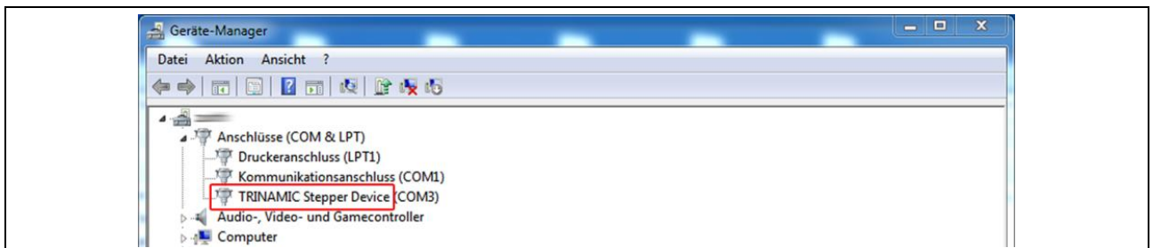
Figure 57: The scanner driver has been installed (the warning sign has disappeared)
