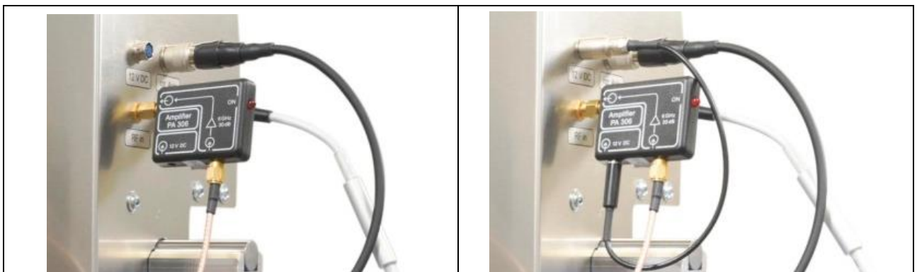
Figure 108: RF measuring cable connected to the preamplifier
