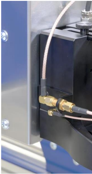
Figure 75: Connecting the SMA-SMA RA measuring cable to the SMA coupling
