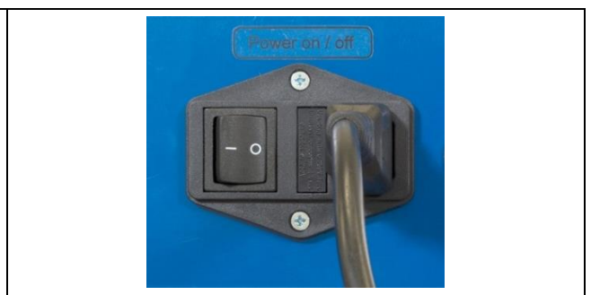
Figure 49: Plugging the power supply plug (C13) into the power supply socket (C14)
