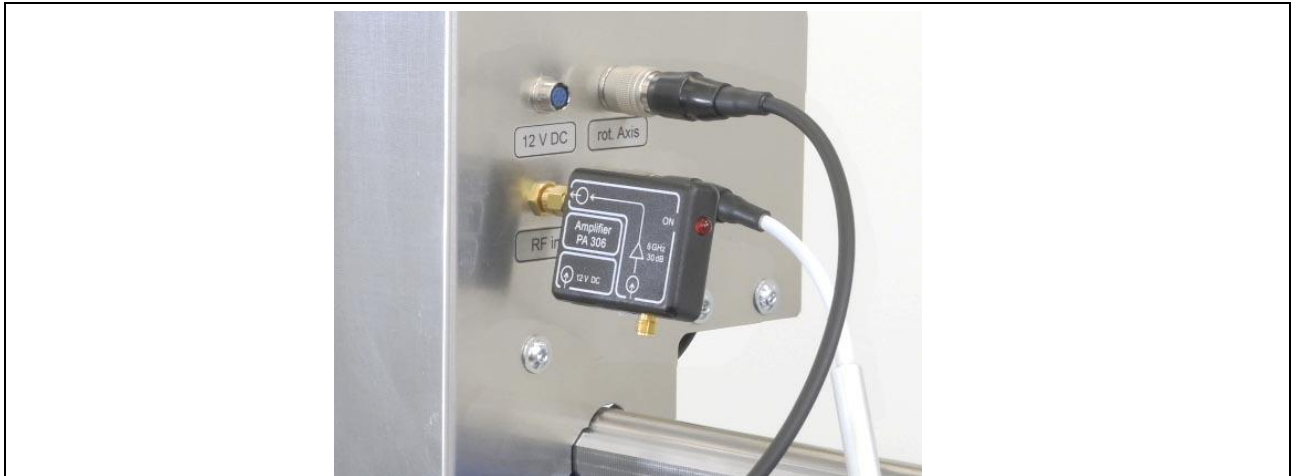
Figure 107: Preamplifier on the input marked RF in on the Z-axis tower
